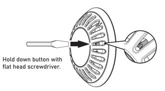
2. While continuing to hold button, rotate counter-clockwise & remove bulb from locking ring.
