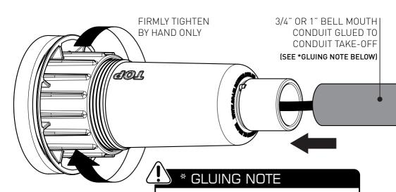
ENSURE P.V.C. SOLVENT CEMENT IS SUITABLE FOR NON-PRESSURE APPLICATIONS AND USE WITH A.B.S. PLASTIC
