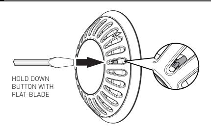
2 ROTATE COUNTER-CLOCKWISE & REMOVE FROM LOCKING RING
