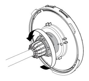
UNSCREW PLUG COLLAR COUNTER-CLOCKWISE UNTIL IT IS FREE SPINNING
