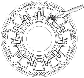
USE A SCREWDRIVER TO LOOSEN THE CAPTIVE SCREW
