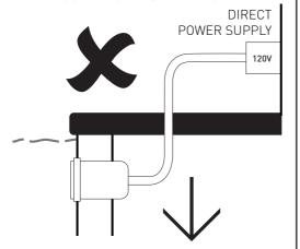
**1B:** A 12V AC TRANSFORMER **MUST** BE INSTALLED BETWEEN THE 120V POWER SUPPLY AND POOL LIGHT
